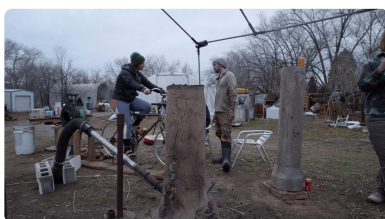
A friend of Cooley's assisting by providing pedal-powered forced air.
